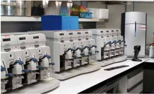
The Affymetrix system at the LSTF 3 Fluidics Stations (left), Scanner 3000 7G with autoloader (right)
