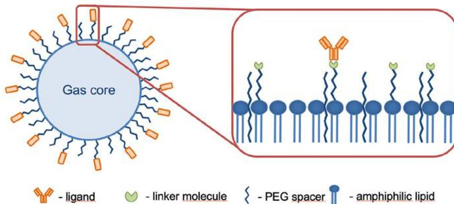
**Fig. 1:** Microbubble contrast agent used for ultrasound molecular imaging. Microbubbles consist of a lipid monolayer shell and a heavy weight gas core. The shell is functionalized with a specific ligand bound to the surface through linker molecules.
