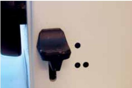
The mechanical trimming device should be used carefully when roughing, particularly the lower (..) setting that produces an advance of 30  $\mu\text{m}$  when activated.
