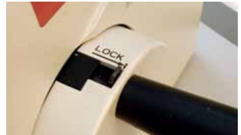
The handwheel lock is shown here with the handwheel in the 12 o'clock position and the lock engaged. This lock will only engage in this position at the top of the cutting stroke.
