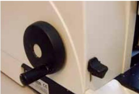
The coarse feed wheel needs to be used carefully when roughing to avoid cutting unintentional thick slices from the specimen surface and causing damage.
